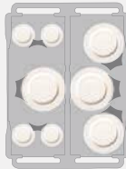
4 columns - plates of \varnothing 115 mm 2 columns - plates of \varnothing 140 mm 2 columns - plates of \varnothing 230 mm
